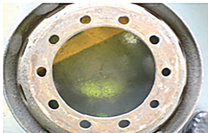
Elongated Stud Holes
