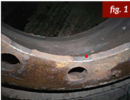
Worn Wheel Bore
