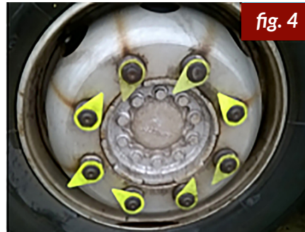
Rust bleed running from the fixing area
