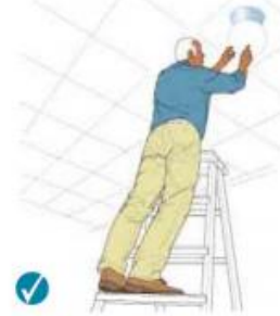
Figure 6b Correct - 3 clear rungs. Don't work any higher up this type of stepladder.
