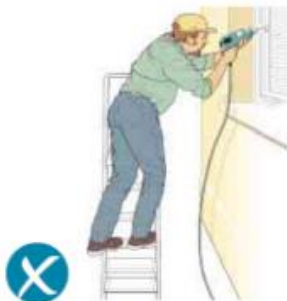
Figure 7a Incorrect - steps side-on to work activity
