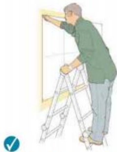
Figure 6a Correct – two clear rungs. Don't work any higher up this type of stepladder.
